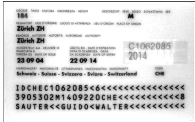
IR absorbing black Ink (under IR light)
