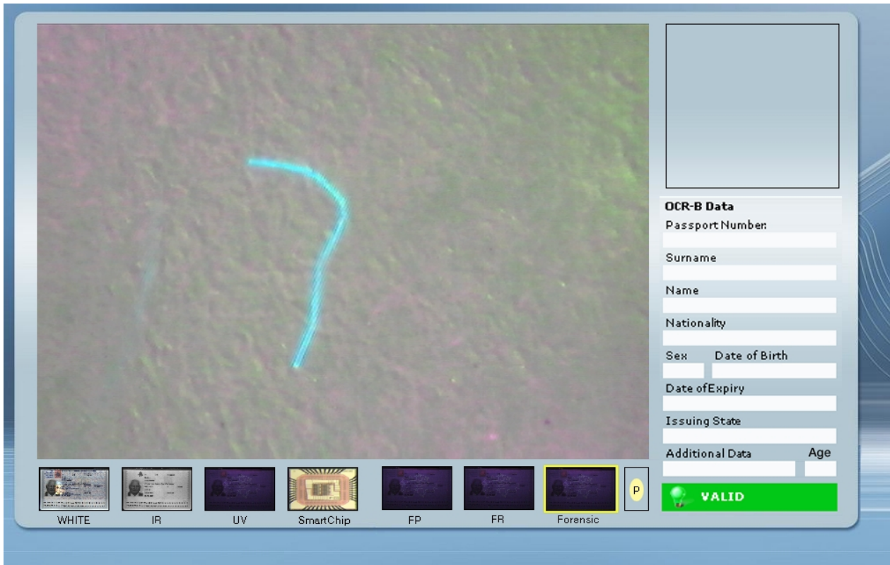
UV fluorescent thread in the Passport paper
