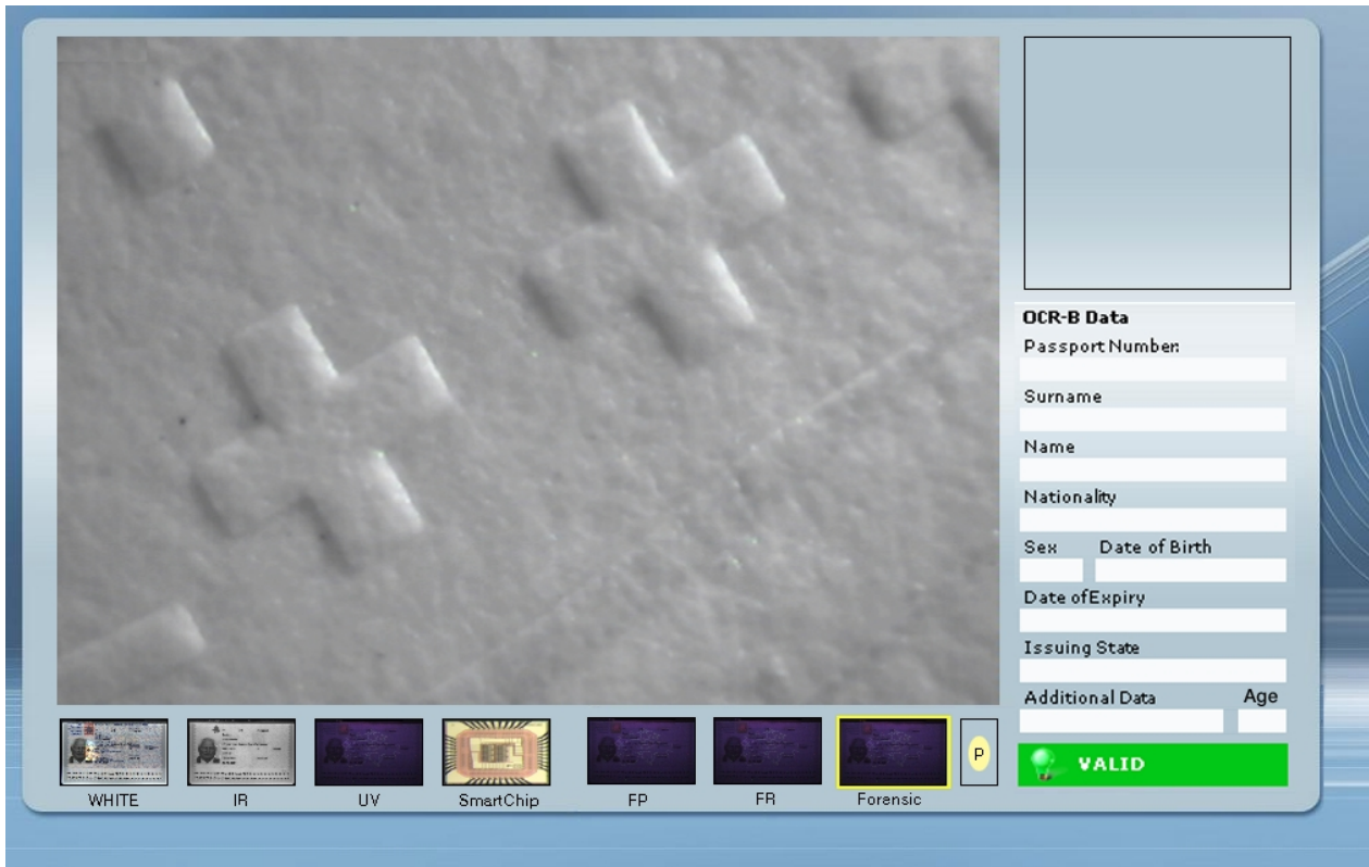
Structure of intaglio printing under IR light
